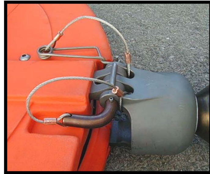
Properly Closed Gate Figure 11
