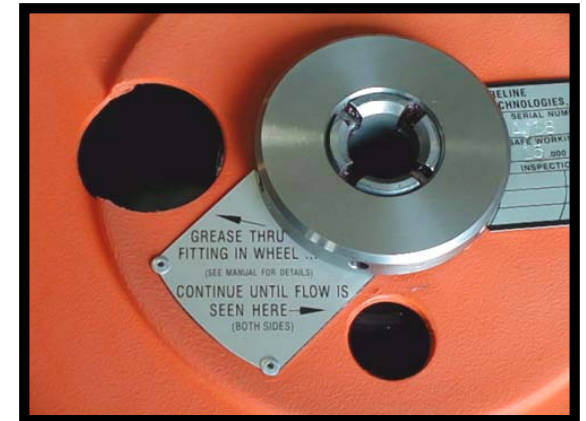
Greasing Holes Figure 12
