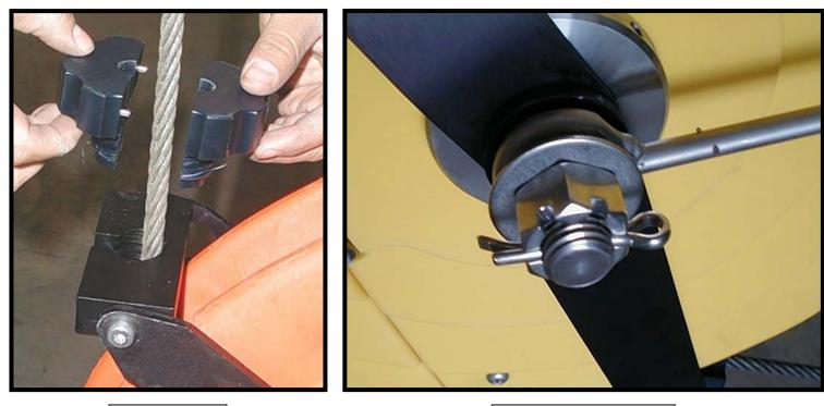
Split Bushing Figure 19 Properly Locked Pivot Pin Figure 20
